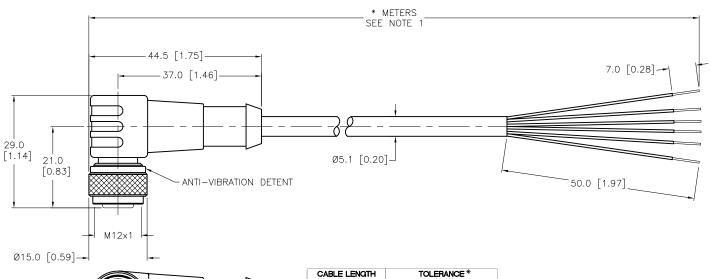
+ 4% (OR 50mm) OF LENGTH - 0% (OR 0mm) OF LENGTH WHICHEVER IS GREATER ALL LENGTHS TOLERANCE \* STRIP LENGTH 0-7mm ±0.5mm 8-29mm ±1.0mm ±2.0mm 30-49mm 50-69mm ±3.0mm 70-100mm ±4.0mm OVER 100mm ±5.0mm \* UNLESS OTHERWISE SPECIFIED
